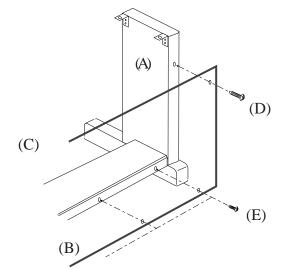
2. Fasten Side Panel (A) and Back Panel (B) with two screws (D). Then fix Back Panel (B) to Pedal Board (C) with four screws (E).
